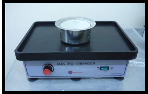
Figure 2: Novolac powder was sieved gently with the aid of vibrator
