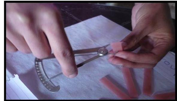
Figure 4: Using of Vernier to standardize the dimensions of each acrylic specimen after finishing
