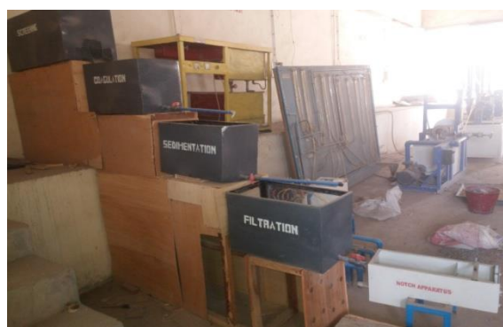
Plate 1: Model water treatment plant
