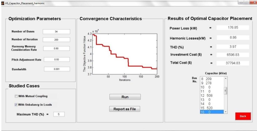
Fig.8: The interface for solving optimal capacitor placement problem
