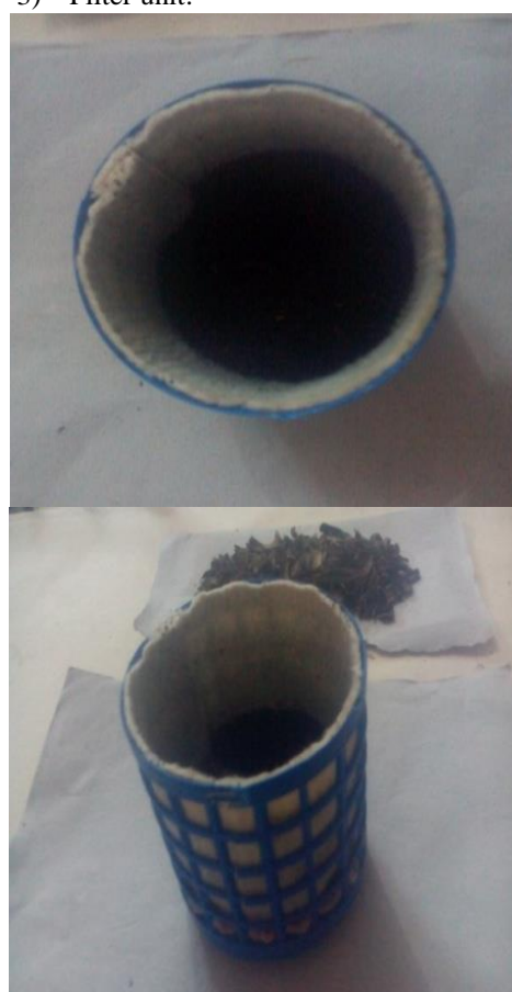
Fig: 3- Filter unit containing banana peel powder.
